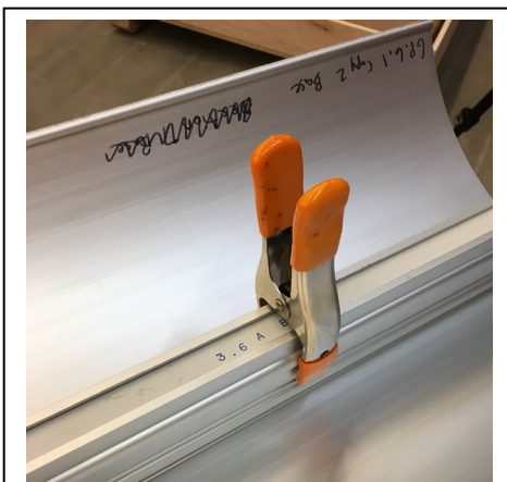
Section 6 bases clamped to the bottom of panel 6.1 so that the bolts and nuts can be attached. Remove clamp after bolting.
